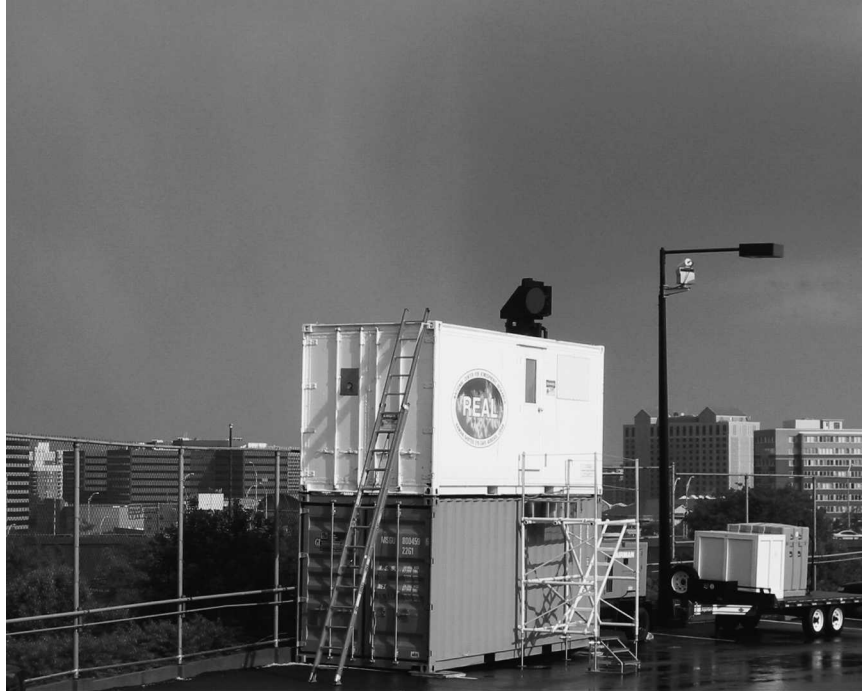
FIG. 4. The top shipping container houses the transmitter and receiver, and the beam-steering unit is installed on its roof. The bottom gray container is an empty shipping container in order to elevate the entire system to obtain a view free from obstructions. Eye safety is imperative for operation in densely populated urban areas.
