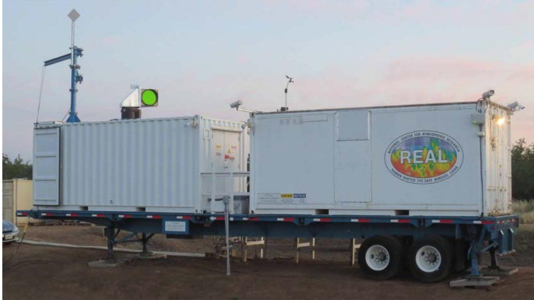
Figure 1. The Raman-shifted Eye-safe Aerosol Lidar at California State University Chico. (Photo taken May 23, 2013.)
