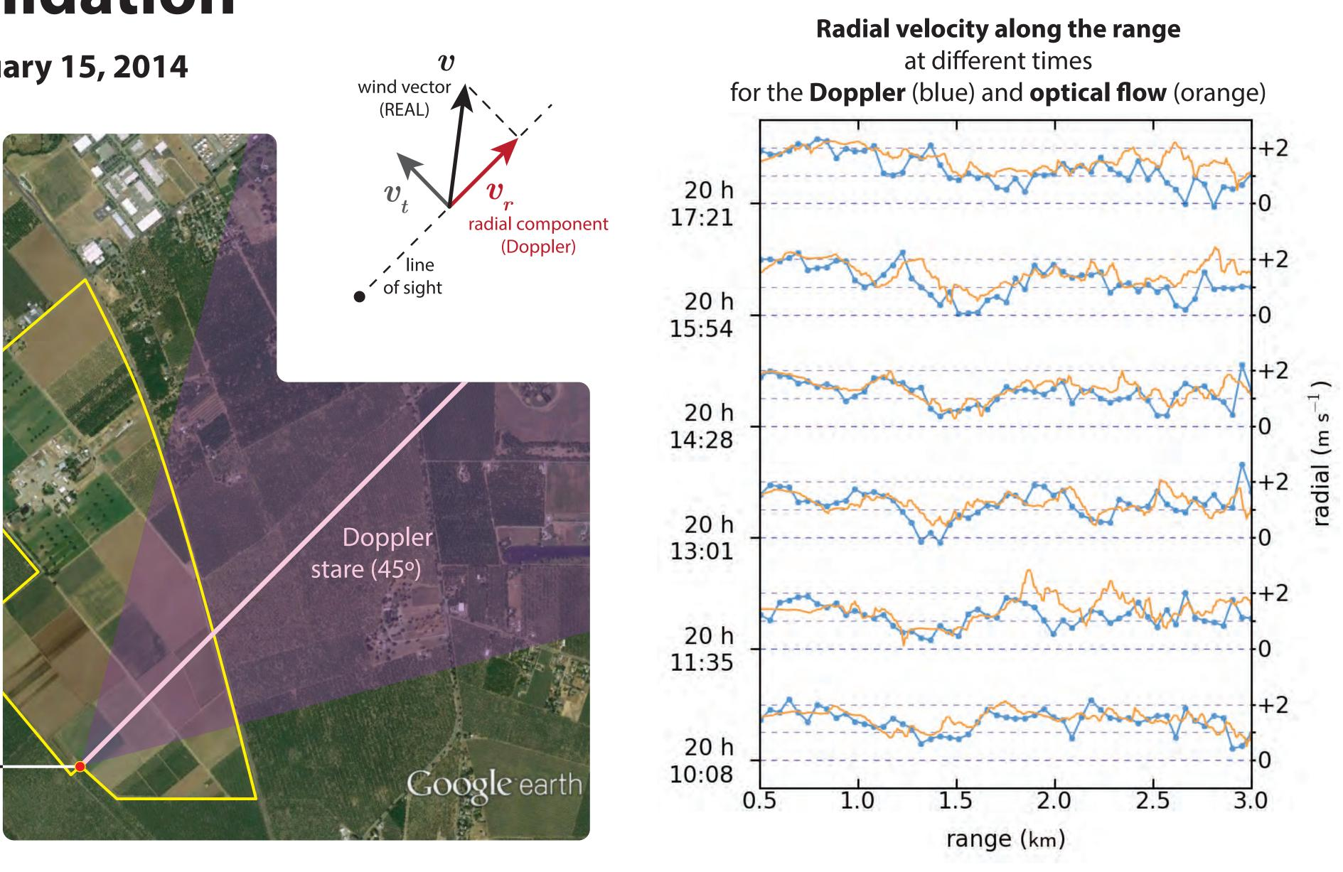
Series of radial velocity as a function of time (horizontal) and range (vertical axis)
