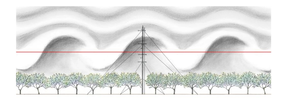
LIDAR: A horizontally scanning aerosol lidar was used to make horizontal cross-sectional images of the canopy waves just above the trees
