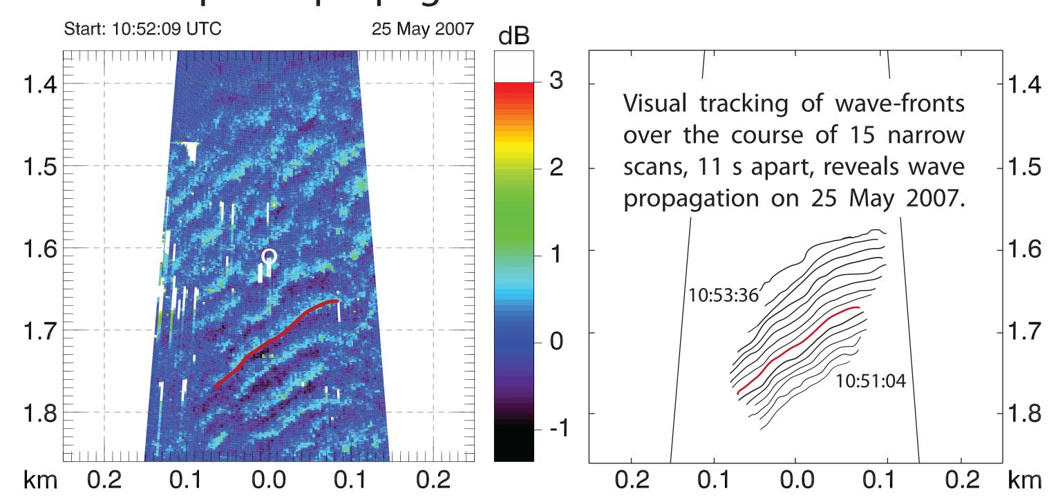
In each case, we can identify the wave-fronts from the lidar scans (above left). Using the visual tracking technique, we can identify the wave phase speed and propagation direction (above right). We can compare these values with values collected from the anemometers on the tower.
