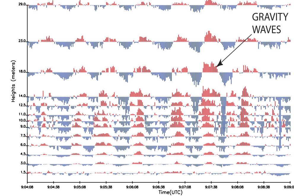
Time series of the vertical wind component show how gravity waves (as observed in the figure above right) can vertically displace the horizontal aerosol strata and enable the elastic backscatter lidar to observe the wave structure in a near-horizontal plane. Coherent oscillations of the vertical component of air motion in the anemometer data support our hypothesis that aerosol strata are displaced by the vertical wind component.
