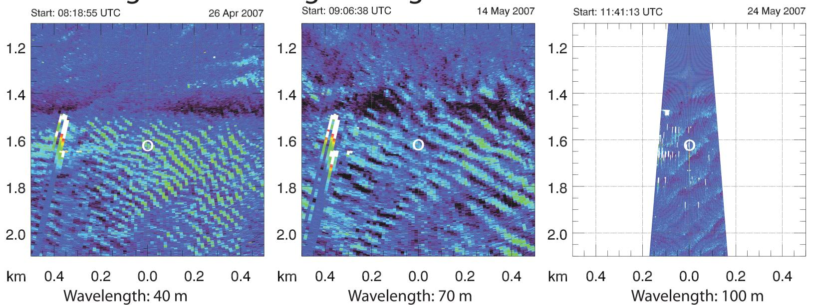
The REAL has the unique capability to measure the spatial extent of these waves. The wavelength is a measurable quantity that can be identified for all 52 cases. The wavelengths range between 40 m (above left) and 100 m (above right).
