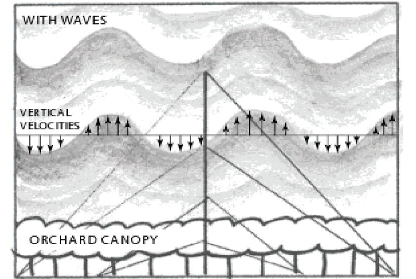
Vertical cross section of the lower atmosphere that may occur at night during quiescent conditions. Stable stratification and weak flow result in the formation of vertical gradients of aerosol backscatter that are horizontally invariant. Perturbations of these strata can form waves.
