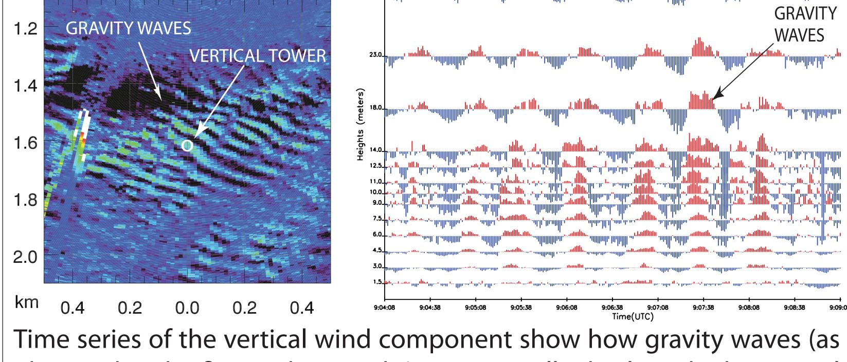
observed in the figure above right) can vertically displace the horizontal aerosol strata and enable the elastic backscatter lidar to observe the wave structure in a near-horizontal plane. Coherent oscillations of the vertical component of air motion in the anemometer data support our hypothesis that aerosol strata are displaced by the vertical wind component.
