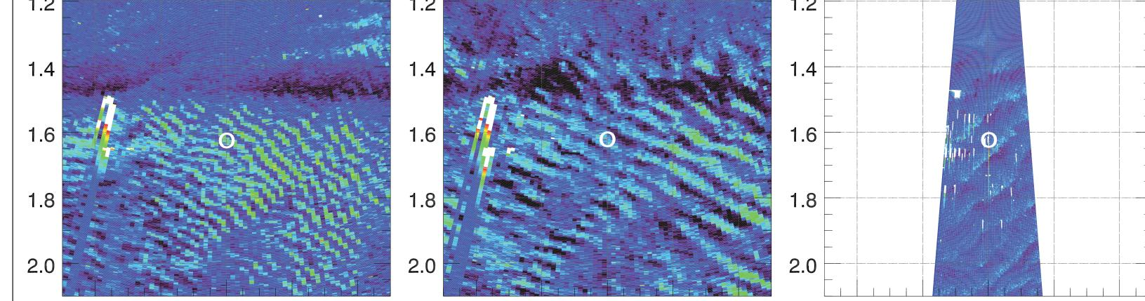
Wavelength: 40 m Wavelength: 70 m Wavelength: 100 m The REAL has the unique capability to measure the spatial extent of these waves. The wavelength is a measurable quantity that can be identified for all 52 cases. The wavelengths range between 40 m (above left) and 100 m (above right).
