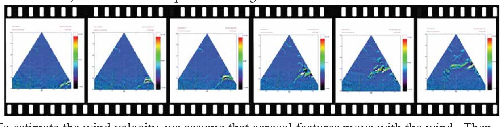
To estimate the wind velocity, we assume that aerosol features move with the wind. Then,
