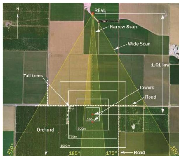
Figure 2. Plan-view of the experimental area. The shaded regions from  $150^{\circ} - 210^{\circ}$  and  $175^{\circ} - 185^{\circ}$  azimuth represent the areas covered by “wide” and “narrow” PPI scans, respectively. The vertical tower (VT) was located 1.61 km directly south of the REAL. The white squares centered on the VT represent the image blocks extracted from the gridded PPI scan data that were used to compute motion vectors via the cross-correlation technique.
