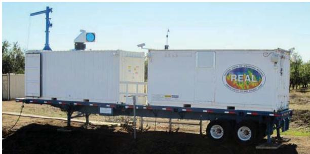
Figure 1: The Raman-shifted Eye-safe Aerosol Lidar (REAL) at the California State University Chico Farm.
