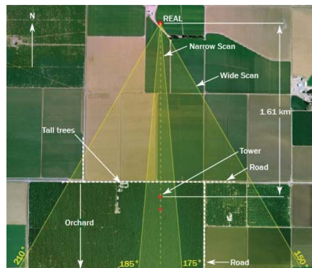
Figure 1. Plan view of the experimental area for the 2007 CHATS. The REAL was located 1.61 km directly north of the 30-m tall NCAR ISFF tower.
