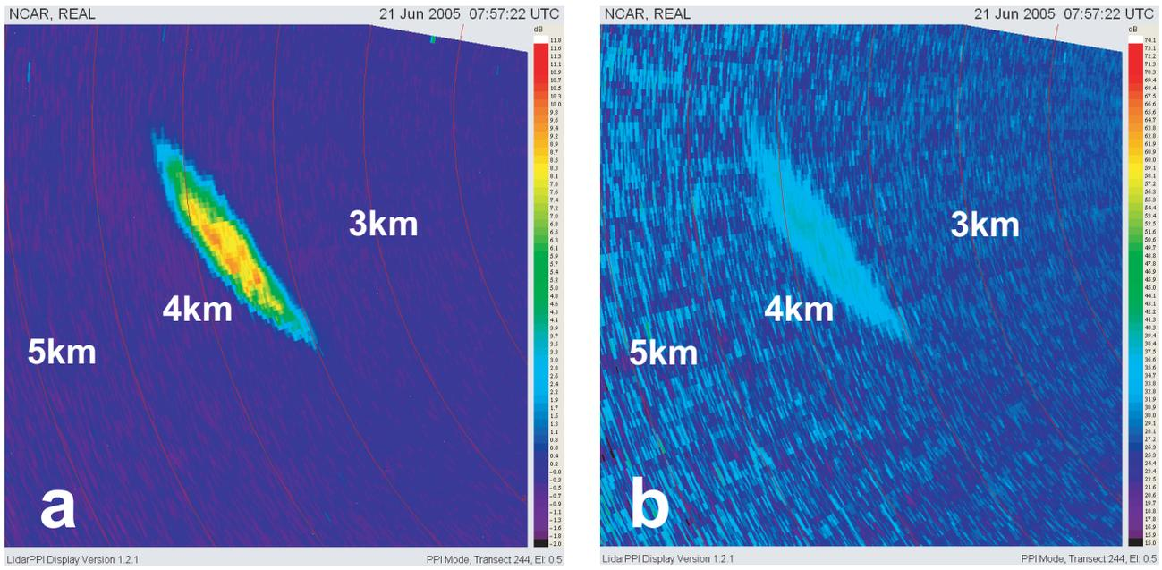
**Figure 7.** (a) Total backscatter intensity (b) Depolarization ratio. 21 June 2005, 7:57 UTC (1:57 LT). A plume of *Bacillus subtilis* var. *niger* (BG) released from an aircraft at 3.5 km range. In this case, the plume had a higher depolarization than the average of the background aerosol (~8% higher.)
