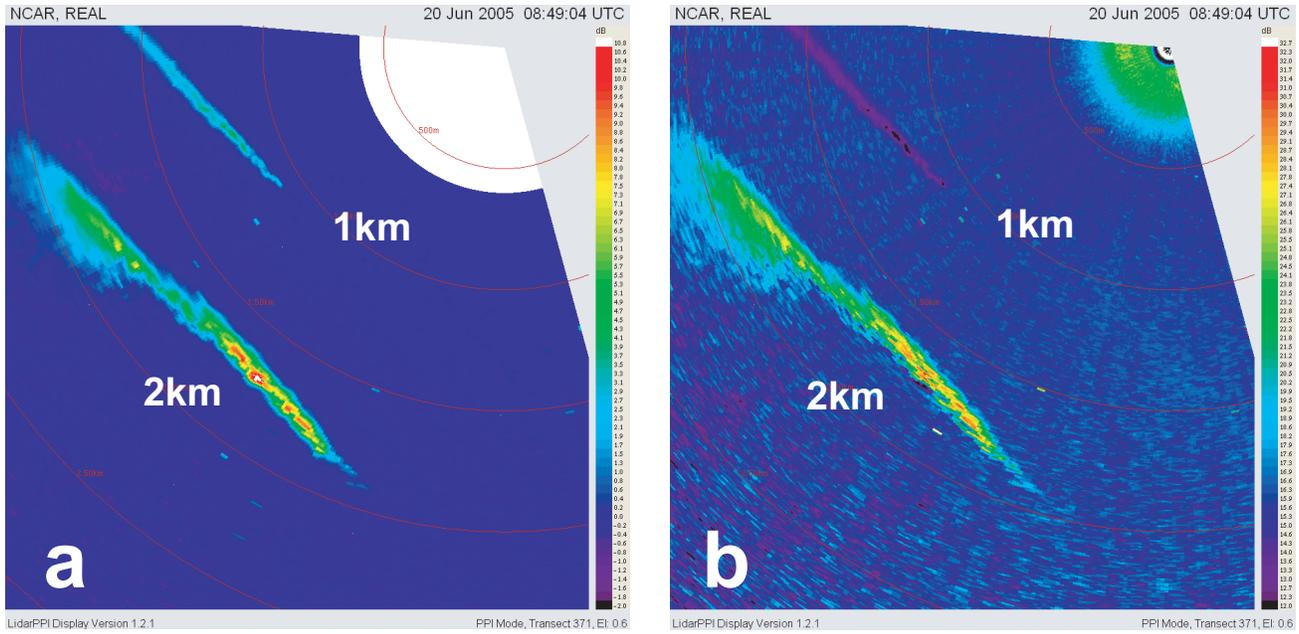
**Figure 9.** (a) Total backscatter intensity (b) Depolarization ratio. 20 June 2005, 8:49 UTC (2:49 LT). The plume that begins near 1 km range is from a point release of male-specific bacteriophage type 2 (MS2, a bacteriophage representative of viral agents) and the plume near 2 km is from an aerial release of BG. The BG resulted in a higher depolarization and the MS2 a lower depolarization than the background aerosol.
