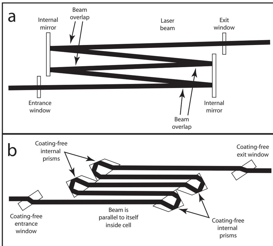
**Figure 3.** Laser beam path through two generations of Raman cells. a) The first generation used windows and mirrors with anti-reflection and high-reflection coatings, respectively. b) The second generation uses optics with surfaces at the Brewster angle and prisms for total internal reflections. Therefore, no coatings are necessary.
