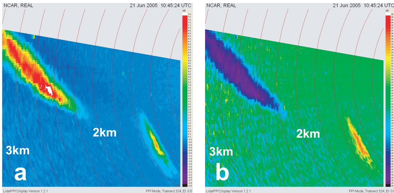
**Figure 6.** (a) Total backscatter intensity (b) Depolarization ratio. 21 June 2005, 10:45 UTC (4:45 LT). The plume between 2 and 3 km range is “white smoke” from a point release and the plume at 1.5 km range is road dust. In this case, white smoke had a lower depolarization while the road dust had a higher depolarization than the background aerosol ( $\sim 11\%$  lower and  $\sim 8\%$  higher, respectively.)
