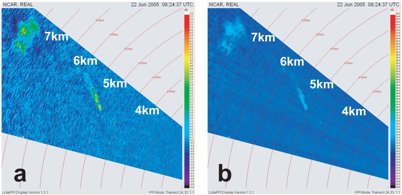
**Figure 8.** (a) Total backscatter intensity (b) Depolarization ratio. 22 June 2005, 8:24 UTC (2:24 LT). The plume between 5 and 6 km range is a gamma-killed vaccine strain of *Yersinia pestis* (YP) and the plume between 7.4 and 7.9 km is road dust. Both clouds have higher depolarization ratios than the background aerosol.
