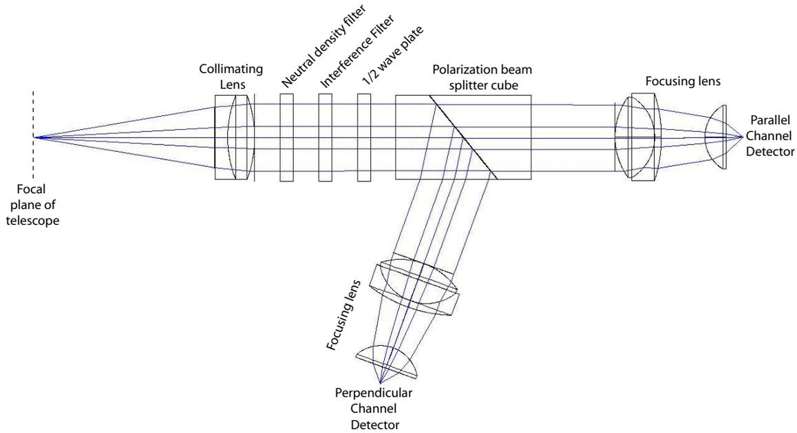
**Figure 4.** Ray trace of the receiver from the focal plane of the telescope to the two detectors.
