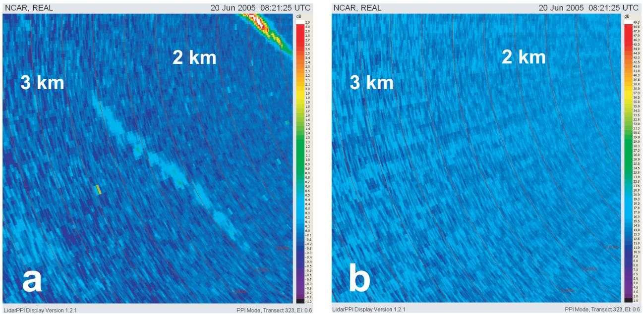
**Figure 10.** (a) Total backscatter intensity (b) Depolarization ratio. 20 June 2005, 8:21 UTC (2:21 LT). The plume in the middle of the image is a low quantity point release of erwinia herbicola (EH) from 2 km range. The plume in the upper right corner of the images is from a high quantity release of the same material. Although difficult to discern, this aerosol type appears to have a depolarization ratio lower than the background.
