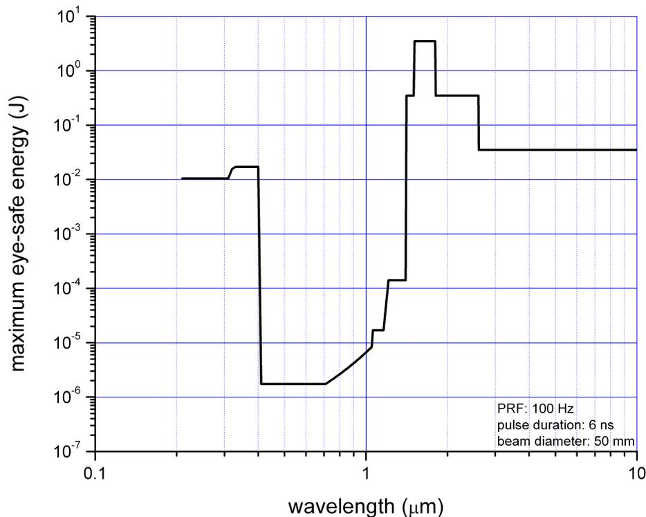
**Figure 1.** Maximum eye-safe laser energy as a function of wavelength for a pulse repetition frequency of 100 Hz, pulse duration of 6 ns, and beam diameter of 50 mm.
