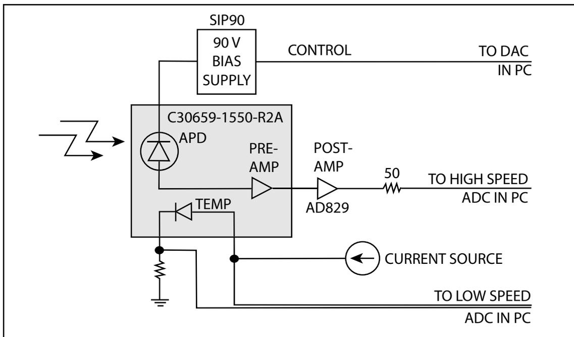
**Figure 5.** Simplified electronics schematic of the detector/amplifier modules used for the data presented in this paper.
