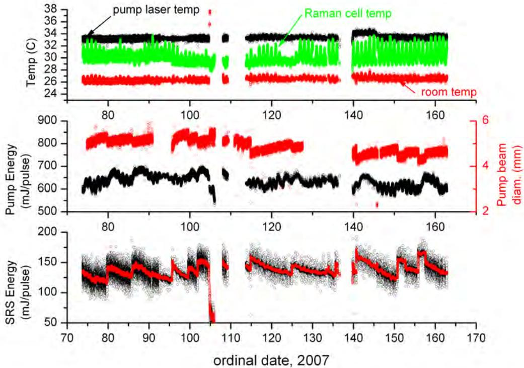
Figure 4. Time series of variables associated with the REAL transmitter during the three-month CHATS deployment.
