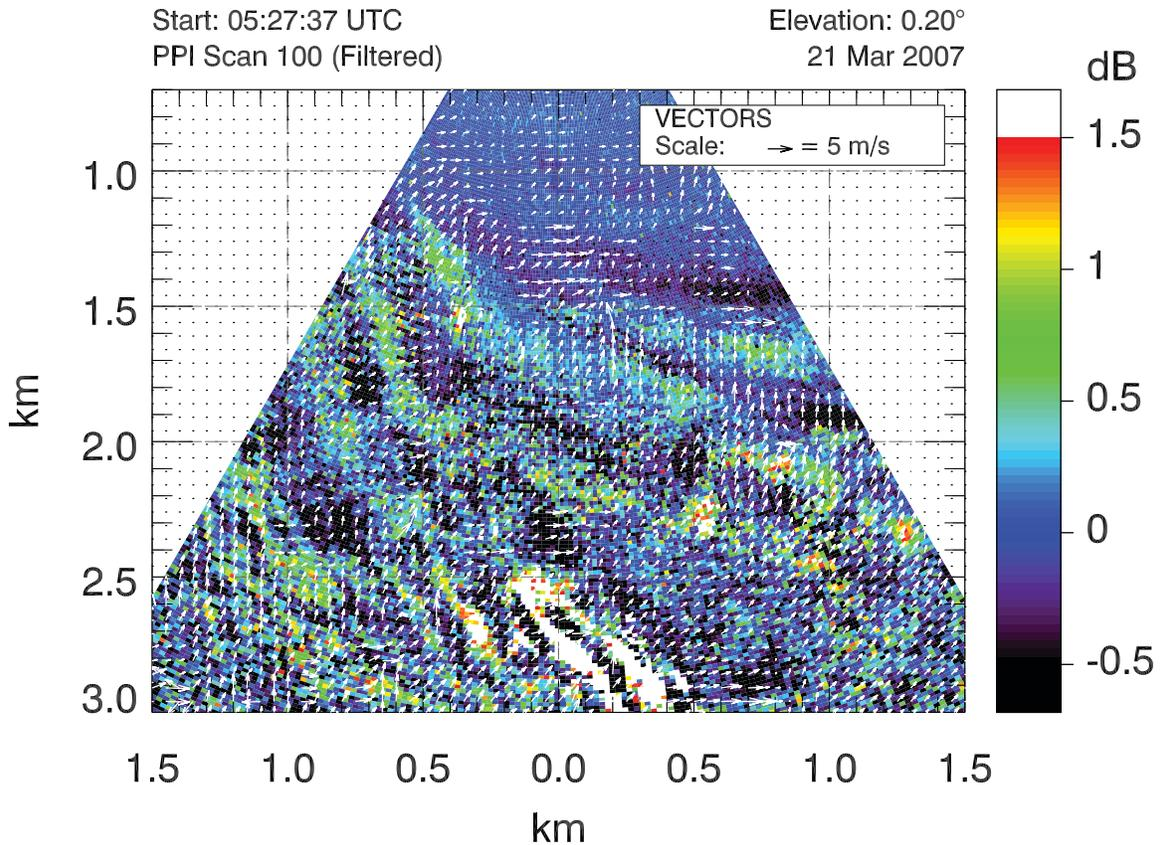
Figure 6. Two component vector flow field for a pair of scans collected on the evening of 21 March 2007. The vectors are spaced every 50 m in x and y and are the result of 250 m x 250 m areas. The vectors are superimposed on one of the two high-pass median filtered backscatter intensity images that were used to compute the vectors.
