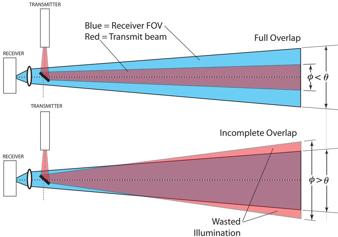
Figure 3. Examples of proper overlap (top) and incomplete overlap (bottom) for an atmospheric lidar system.
