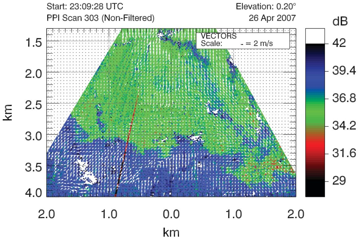
Figure 8. Two component vector flow field for one pair of scans collected on 26 April 2007. The vectors are spaced every 50 m in x and y and are the result of 500 m x 500 m areas. The vectors are superimposed on one of the two high-pass median filtered backscatter intensity images that was used to compute the vectors. The color scale of the backscatter data has been adjusted so that the advancing marine airmass is blue and the airmass north of it is green.
