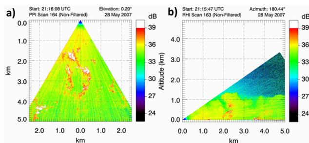
Fig. 2: a) Horizontal and b) vertical lidar scan showing aerosol plumes over a walnut orchard in Dixon, CA on May 28, 2007.
