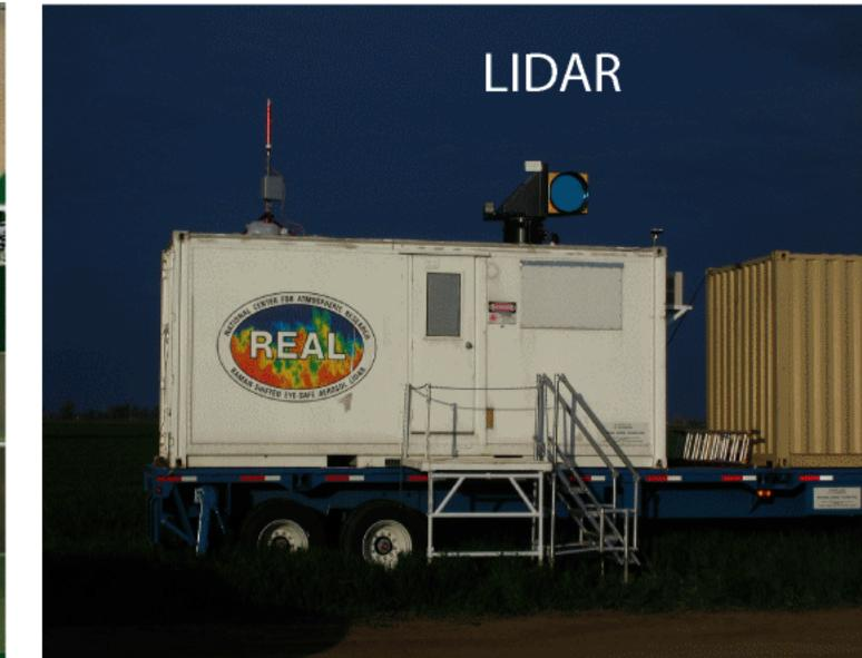
Sonic anemometers on the tower (left) sample 3-component wind velocities at 60 Hz. The lidar (right) scans over the orchard and through the tower at about 18 m altitude. Time-series data from the anemometers can be used to determine the period of the waves. Lidar scan images can be used to determine the wavelength of the waves. If the lidar scan images are collected rapidly enough, phase velocity can also be measured.
